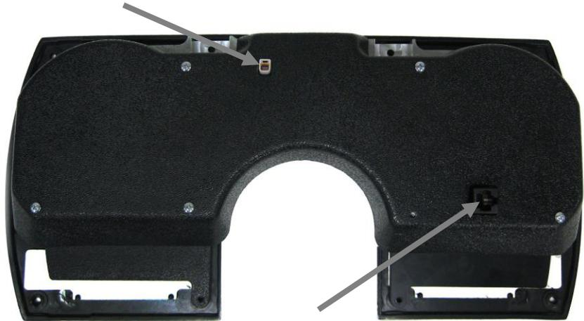
5b. Connect the CAT5 cable to the system so it can be routed and connected to the control box as the system is re-installed.
