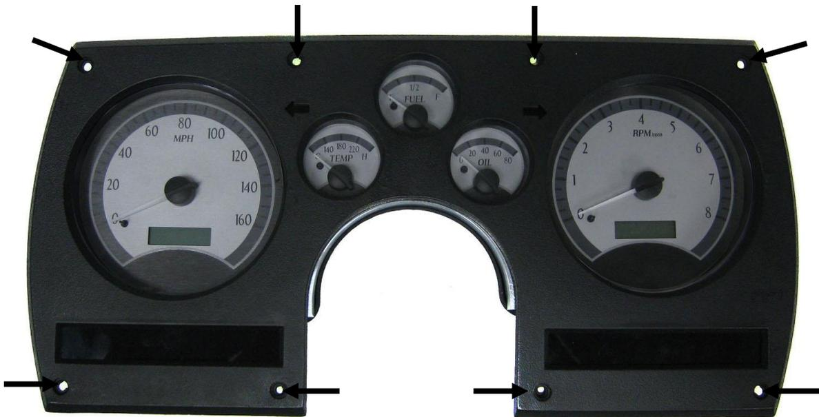
6. Secure the VHX system and the bezel back into the dash using the eight original screws. Refer to the main manual for wiring instructions to complete the VHX installation.
