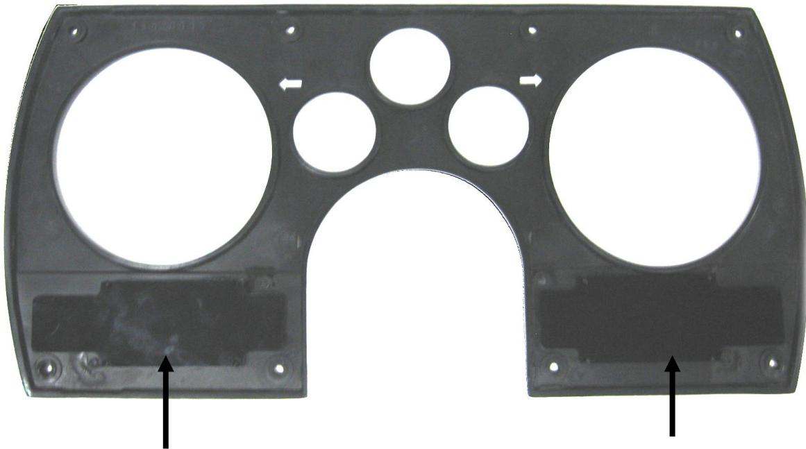
4a. Remove the protective tape from the clear lens and install the VHX system into the bezel. Watch carefully as you insert the system so you don't scratch or damage the lens.
