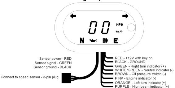
\*To avoid damage to motorcycle, please see Speedometer and Indicators sections for details on locating VSS and indicator wires for most motorcycle applications
