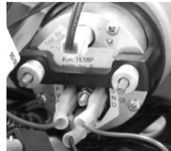
Connection shown with optional spade terminals
