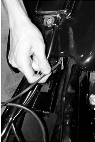
Route wire under tank
